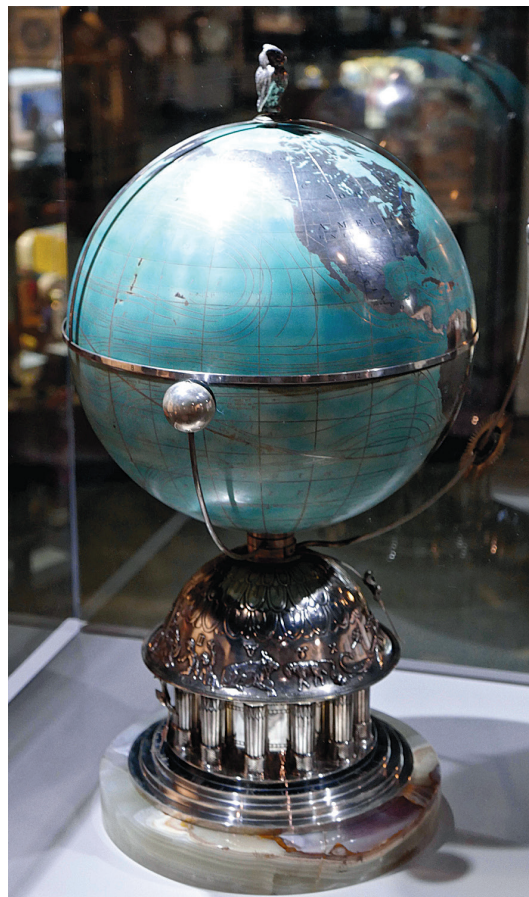
Now owned by the NAWCC museum and currently on exhibit there, this globe clock was donated to the James Arthur collection in 1956 by Mrs. Harold L. Chalifoux (1895-1987). Its case is sterling silver with turquoise enamel; its base is onyx. The astronomical movement is inside the silver dome beneath the globe that revolves on its axis once every 24 hours. Its indicators, when properly situated, can tell the time of day and date anywhere in the world. It was made by Tiffany’s own clockmakers and jewelers for display at the World’s Columbian Exposition in Chicago in 1893. “I am so glad that I have found a proper home for this very magnificent clock which I have grown up with since childhood,” the donor wrote to Edward C. Smith, the Arthur collection curator at the time. She was obviously under the impression that the clock would be at NYU forever. Asked about its current value, a New York auction-house specialist kindly replied via e-mail: “The clock is fully described in Tiffany’s catalog of its exhibit at the World’s Fair. Based on that, I would say informally that it would easily fetch at auction a sum in the low to mid six figures.” Schinto photo.
